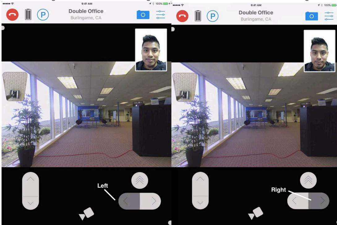
4. The camera icon on the bottom center of the screen will expand the downward facing camera (Always on the Floor View only capable with [Camera Kit](#)). This is perfect for navigating tight spaces or for parking in the charging dock.
