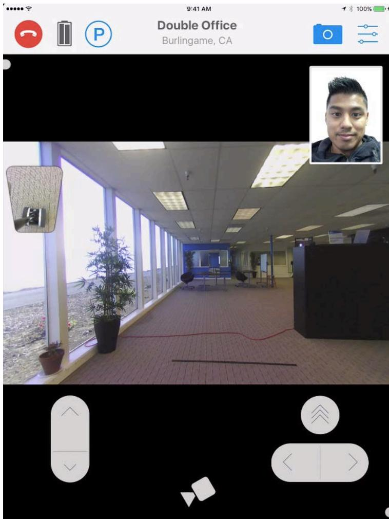
2. The up/down buttons on the lower left hand side, will move your Double forward and backward.
