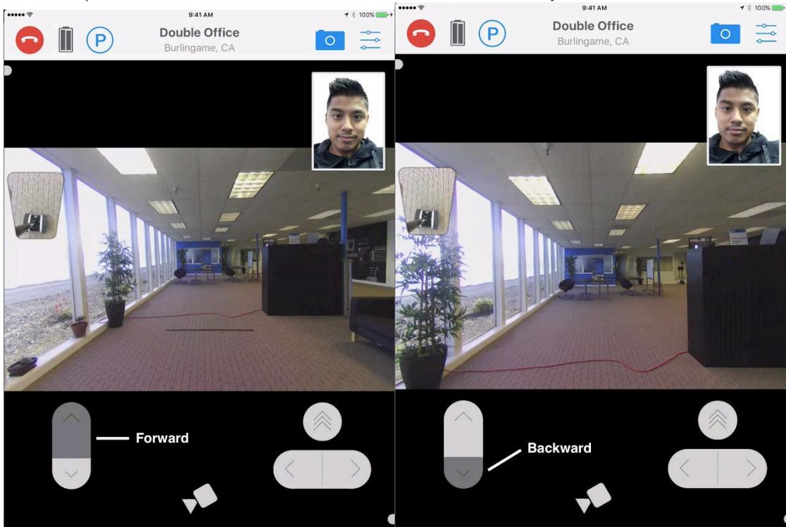
3. The left/right button on the lower right hand side will turn the Double left or right.
